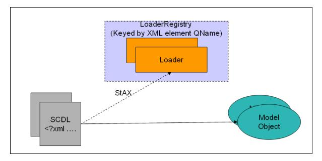
To partipate in the loading process, an extension should provide a component that implements the <u>StAXElementLoader</u> interface and should register that component with the framework's <u>StAXLoaderRegistry</u> during initialization.
