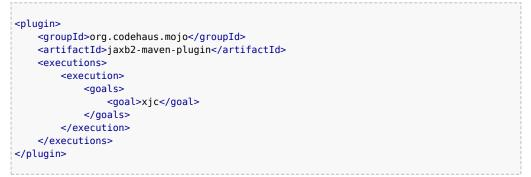
That should do it (it automatically looks for XML Schemas in src/main/xsd to generate beans for). Run **mvn install** and it should emit the beans into target/generated-sources/jaxb. Your IDE should see them there, though
